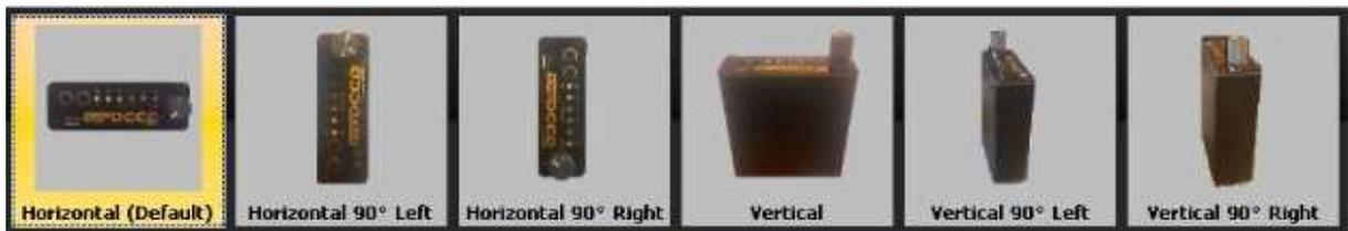
Please select your mounting position from the software options provided and run the accelerometer calibration function as confirmation.
