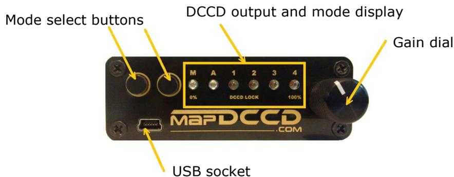
**Mode select** The mode select buttons are used to click through the operation modes of the MapDCCD controller in the left or right directions. The operation modes are ordered: Manual, Auto, Map 1, Map 2, Map 3, Map 4. When a mode select button is pressed, the MapDCCD controller will beep and the LED corresponding to the operation mode will flash rapidly before reverting to show the live output.
